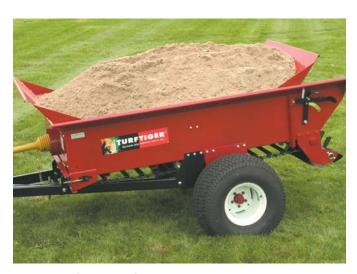
The loading flares simplify loading, add to the capacity and help prevent spills during transport.
