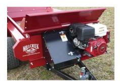
**OPTIONAL Engine Drive**13hp Honda engine with drive remote control electric clutch
