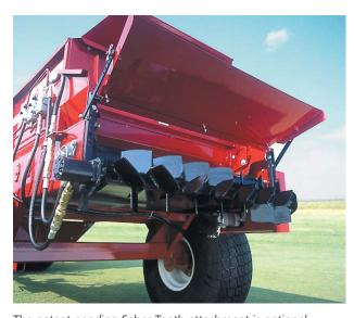
The patent pending Saber Tooth attachment is optional equipment on the Turf Tiger 4300 It is remarkably powerful, yet applies a consistent and uniform spreading pattern that ranges from 8' to 12' wide, depending on the material.
