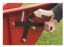
**Metering Gate**Easily adjusts for high volume material flow to the Saber Tooth beater.
