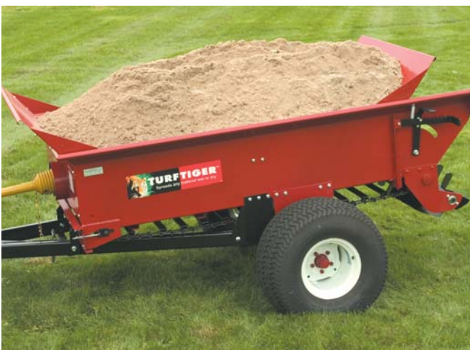
The loading flares simplify loading, add to the capacity and help prevent spills during transport.
